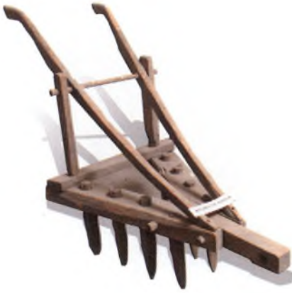
(Above) Pictured here is a handmade harrow. It was used to cultivate cotton.
