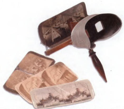
(Above) This is a stereoscope from the 1890s. It was an early form of 3-D viewing.
